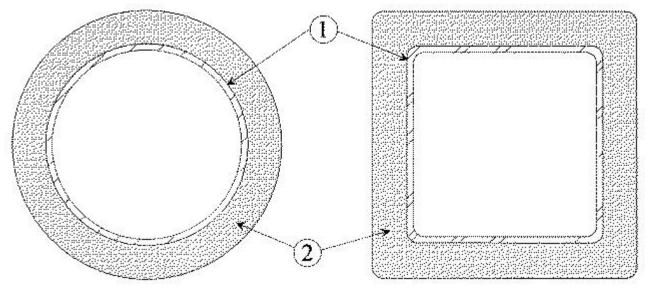
1. **Steel Pipe or Tube Column** — Steel circular pipe (SP) or steel square or rectangular tube (ST). The A/P ratio of the steel pipe or tube (see Item 2) shall range from 0.18 to 2.0.
